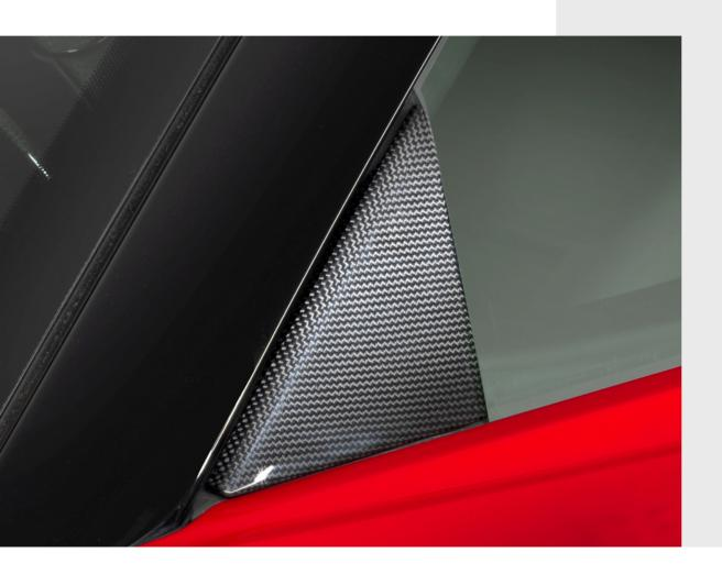
The carbon fibre window triangle trim lets owners personalise their Ferrari with an extra touch of exclusiveness, while the inherent lightness of the material contributes to reducing the overall weight of the vehicle. The distinctive look of carbon fibre accentuates the sports spirit of the vehicle, complementing the exterior design without altering the signature style of the car.
