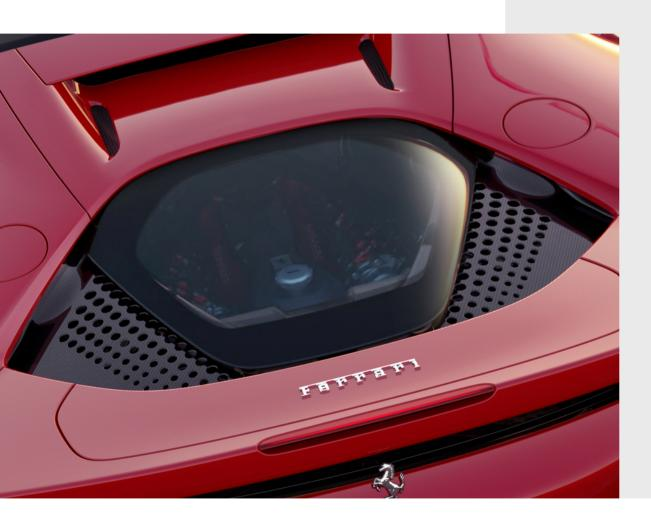
The covers, installed in the end area of the rear window ensure, through their particular shape, the correct air flow of the engine compartment.
