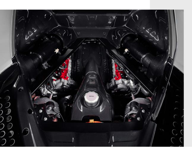
The carbon fibre engine compartment shields are lighter than the standard parts. Carbon fibre is an ultralight, heat resistant material that is also durable thanks to its technical and aesthetic properties and the clear protective layer that covers it.
