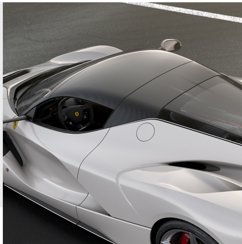
Hard-Top, in naked weave carbon fibre
