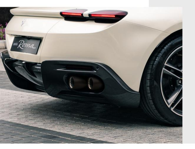
The steel tailpipe tips with a ceramic coating use innovative materials and have specific surface treatments which give the vehicle a tougher, sportier look. The ceramic coating is able to disperse a great deal of heat, withstand accidental damage and, thanks to the special technology used, preserve the same appearance for years.
