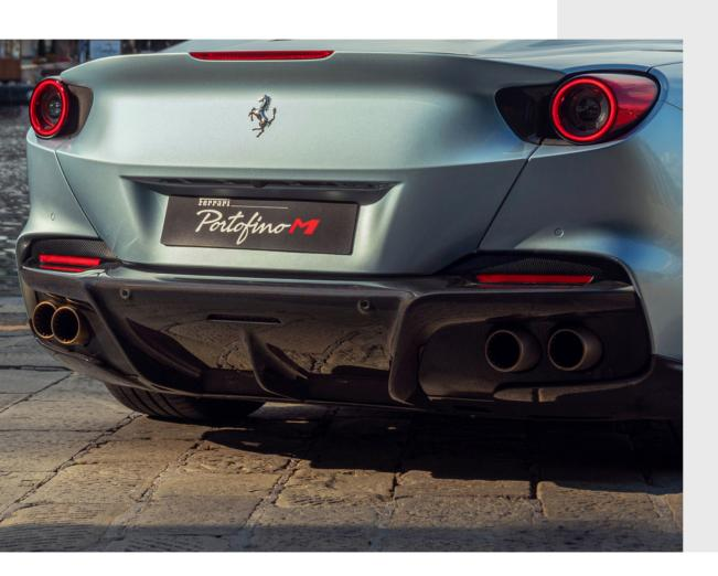
Designed to increase rear downforce and facilitate the evacuation of air from the underbody, the carbon fibre diffuser accentuates the style of the car while performing a precise aerodynamic function and contributing to reducing weight.
