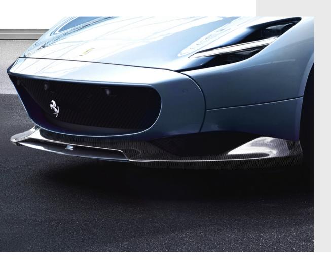
Developed with advanced fluid dynamics modelling technology and honed in the wind tunnel to optimise underbody aerodynamics, the carbon fibre front spoiler performs a crucial function for overall aerodynamic performance while offering the customer an opportunity to personalise the looks of their vehicle.
