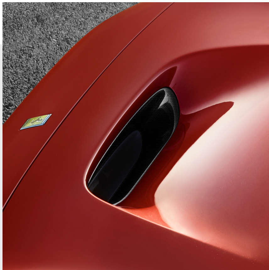
Carbon fibre front spoiler, front S-Duct
