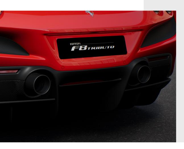
The steel tailpipe tips with a ceramic coating use innovative materials and have specific surface treatments which give the vehicle a tougher, sportier look. The ceramic coating is able to disperse a great deal of heat, withstand accidental damage and, thanks to the special technology used, preserve the same appearance for years.
