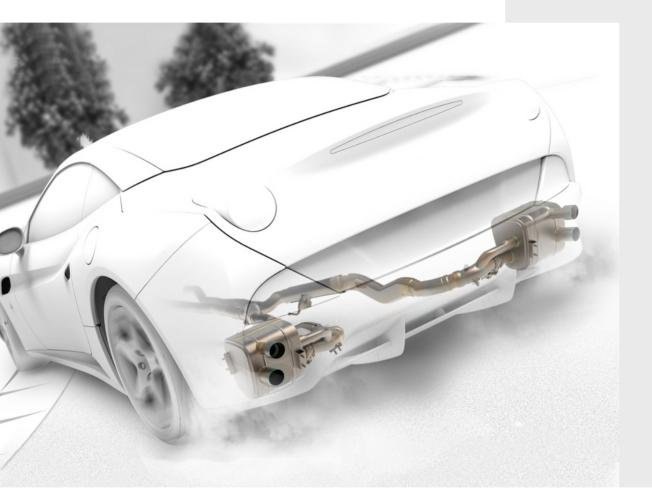
The road legal silencers accentuate vehicle sound thanks to optimised volume of the components and offer the driver a sportier feel. The configuration has been tested and guaranteed by Ferrari and installation requires no modification to the ECU since the new component has been integrated into the standard exhaust range.
