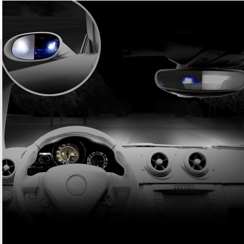
Electrochromic mirrors, exterior
