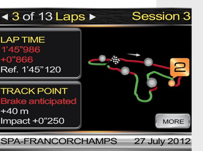
The Ferrari Telemetry Kit - which is integrated in the multimedia system - monitors the position of the vehicle and analyses and records performance data for each track session. The key parameters recorded may then be viewed directly on the dashboard or on an iPad device or PC.
