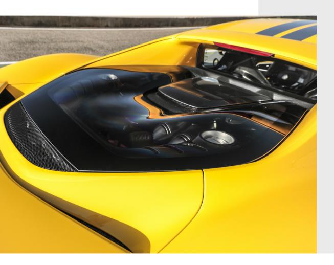
Lexan rear screen further reduces car's weight about 3 kg and makes the engine more visible as is more transparent. This option definitely enhances the racing DNA of the car.
