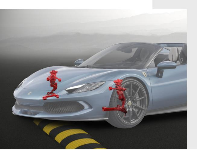
To guarantee maximum performance in any driving situation, Ferrari Genuine offers a system that makes it easier to drive over bumps or ramps and avoid damaging the vehicle. The lift system, which acts on the shock absorbers, lifts the vehicle approximately 40 mm.
