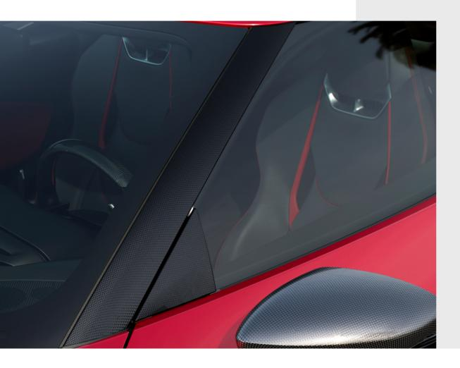
The carbon fiber A-pillars, exclusively made for the Accessories catalog, lend uniqueness and exclusivity to the 296GTB and help to reduce its overall weight.
