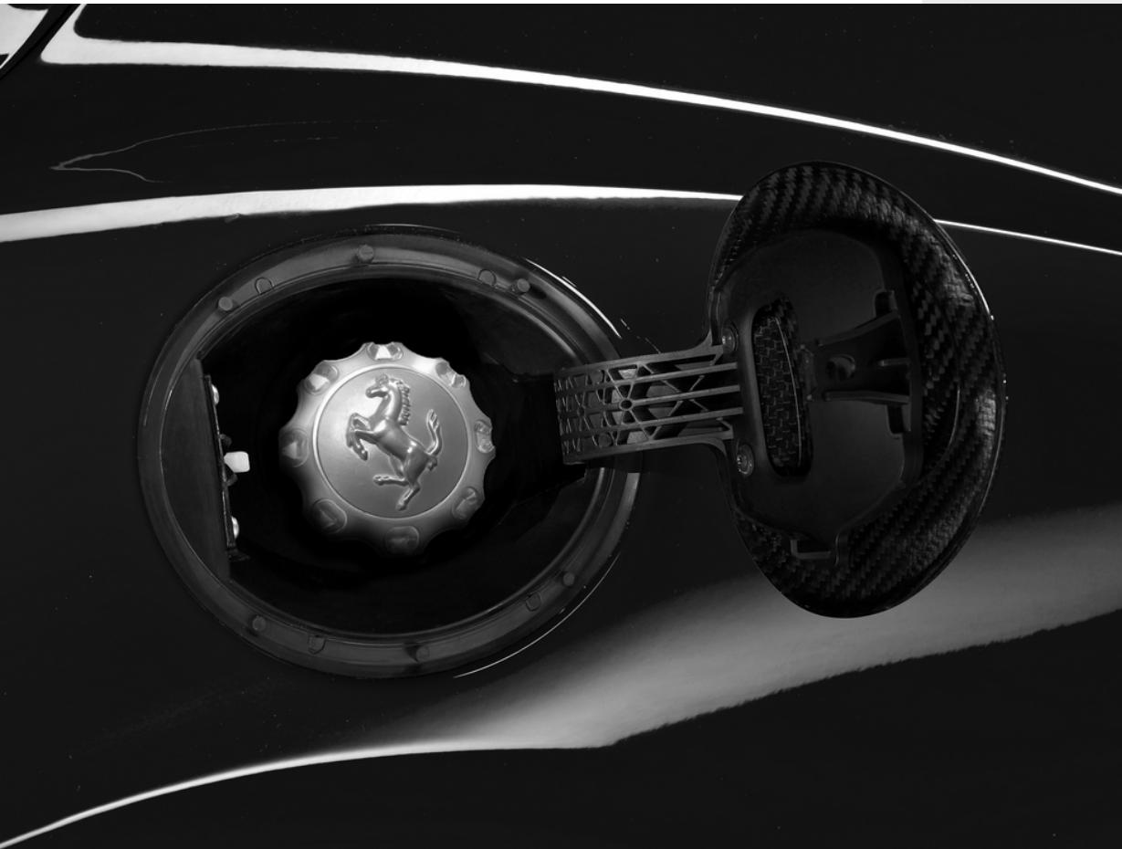
The technology and materials used to make the titanium fuel cap come directly from Ferrari's experience in the world of racing. The cap is forged and then precision-machined and the Prancing Horse logo is laser engraved.
