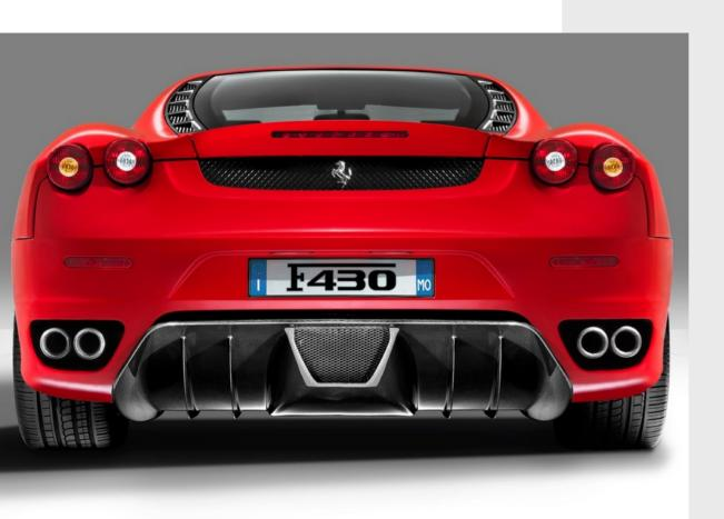
Designed to increase rear downforce and facilitate the evacuation of air from the underbody, the carbon fibre diffuser accentuates the style of the car while performing a precise aerodynamic function and contributing to reducing weight.
