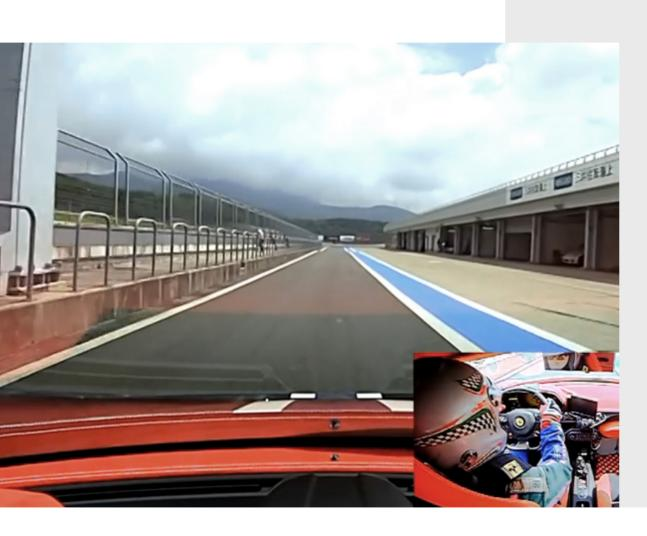
The track cameras are an optional accessory orderable in addition to the Ferrari telemetry kit. When installed in the passenger compartment, and positioned to film both the circuit and the driver zone, these cameras let drivers record their driving experience and review their performance afterwards in high definition video and analyse driving line, braking points and driving technique.
