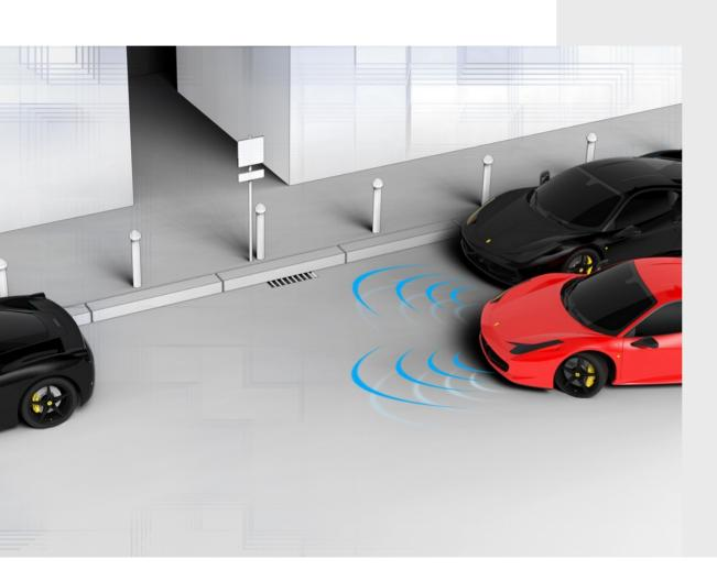
The parking sensors designed by Ferrari indicate the presence of obstacles in front of or behind the vehicle by emitting an acoustic alarm and provide the driver with information on how far away the obstacles are. These sensors help the driver to avoid accidental contact when manoeuvring by combining direct visual information with the acoustic and visual information generated by the system.
