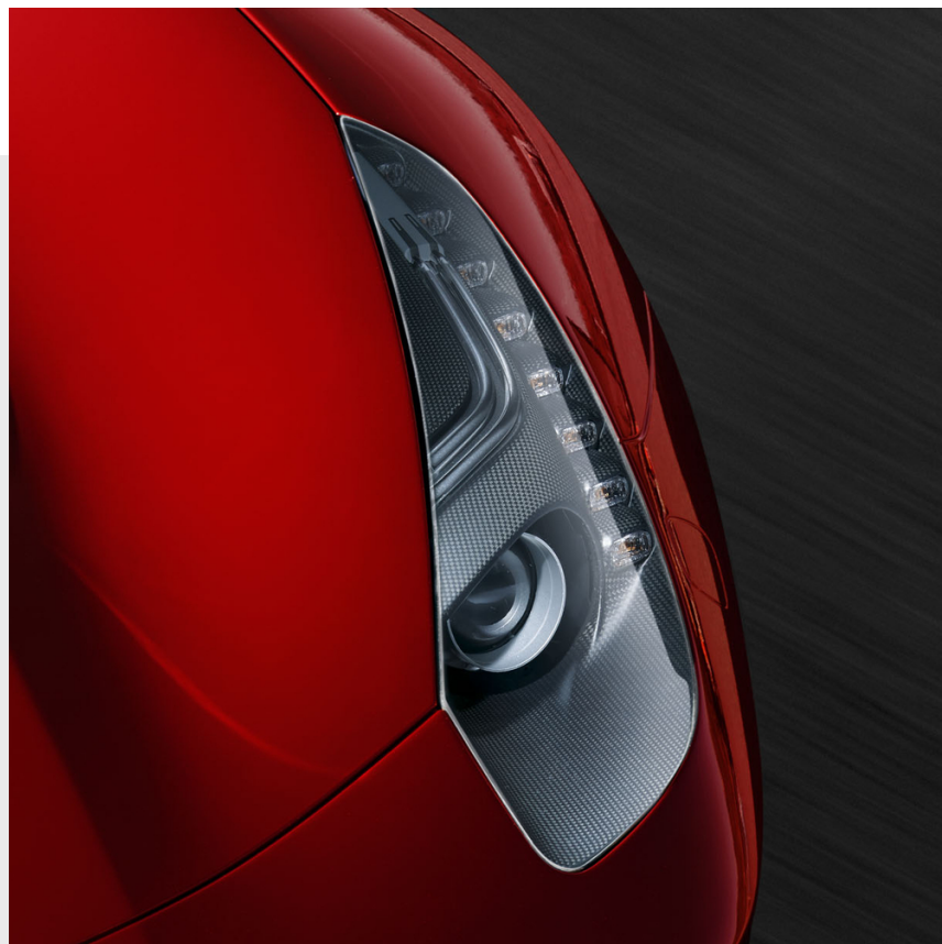
Carbon fibre headlamp tubs, AFS
