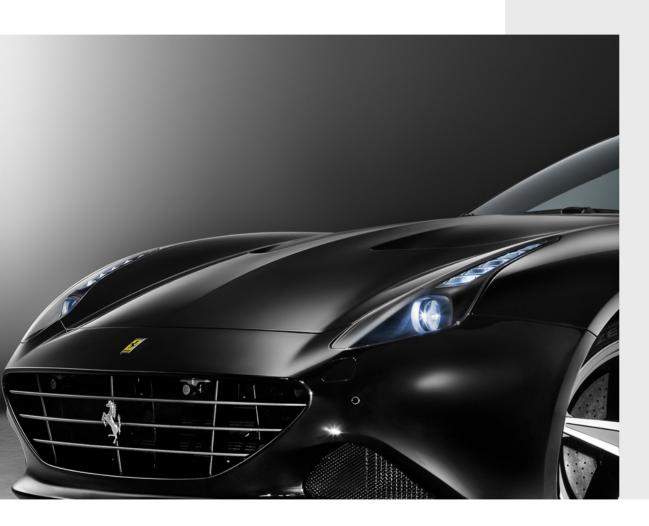
To guarantee a better driving experience as far as safety and performance are concerned, the Genuine accessories catalogue offers customers the chance to install Advanced Frontlighting System (AFS) headlights which direct the beam according to the direction of the bend, optimising the light intensity and improving visibility.
