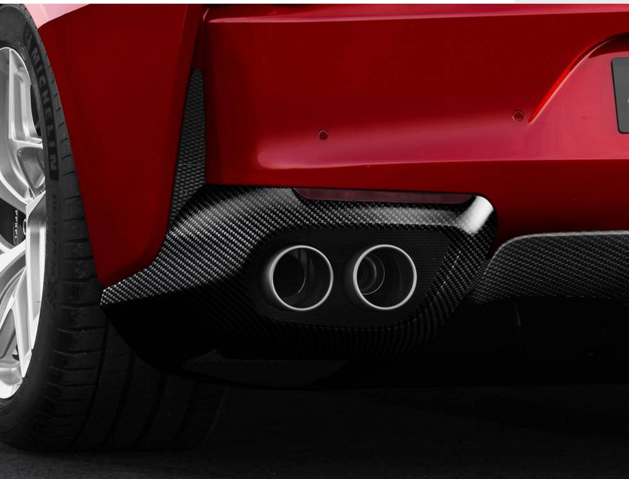
Designed to increase rear downforce and facilitate the evacuation of air from the underbody, the carbon fibre diffuser accentuates the style of the car while performing a precise aerodynamic function and contributing to reducing weight.
