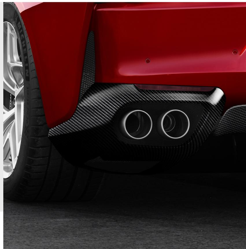
**Carbon fibre rear diffuser**
