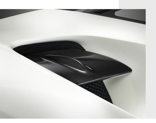
The splitters fitted in the side air intakes are iconic elements that characterize the sporty lines of the car, as well as separate the air flows to ensure maximum engine performance,
