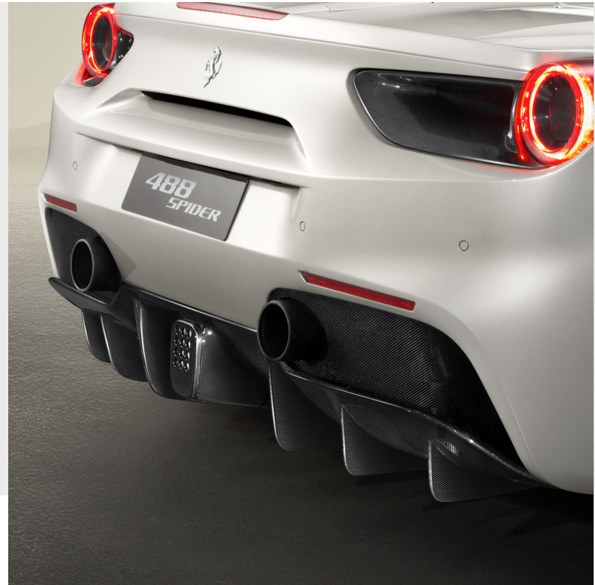
Carbon fibre rear diffuser, rear analogue camera
