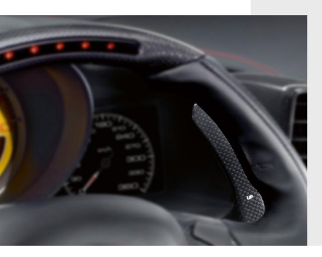
The F1 paddles behind the steering wheel can be replaced with a paddle kit made entirely of carbon fibre.
