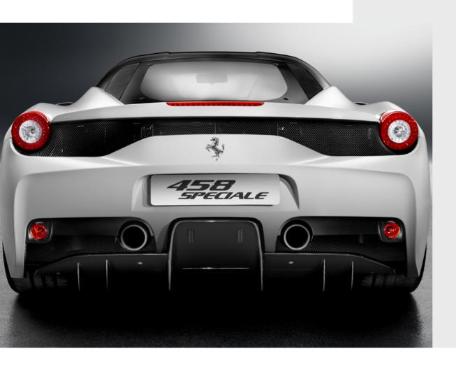
The carbon fibre aerodynamic flaps make a strong aesthetic impact and help to reduce the vehicle's overall weight.
