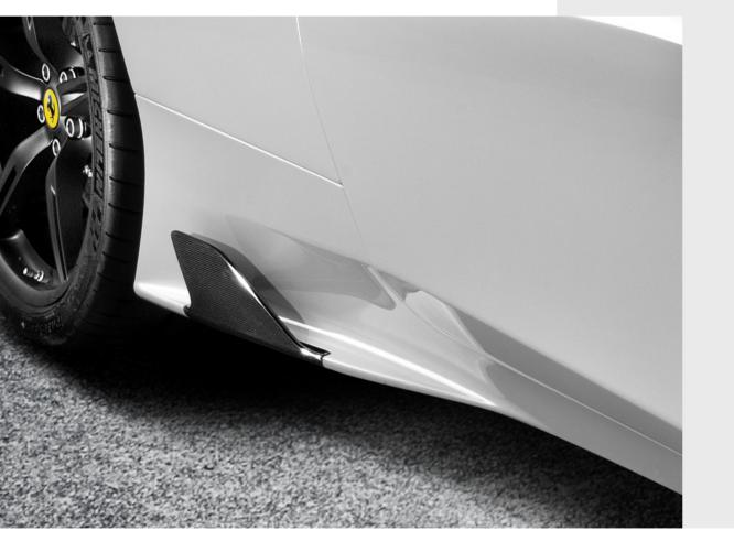
The aerodynamic fins are the side view's most distinguishing characteristic.
