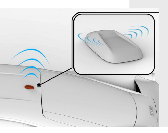
With innovative SDARS (Satellite Digital Audio Radio Service) technology, Ferrari offers a compact high performing product with low visual impact that is able to integrate multiple services.
