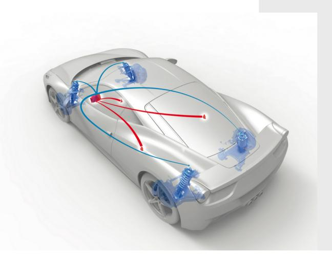
The HS kit introduces new content developed to enhance the sports character of the vehicle for even more intense driving pleasure on the road. The new performance content introduced with this kit includes innovative new magnetorheological shock absorber control software, which increases yaw-pitch-roll damping quality and improves tyres performance for an even sportier steering feel. This control function is active in all manettino positions with specific calibrations for each.
