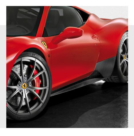
Carbon fibre under-door kit, full carbon
