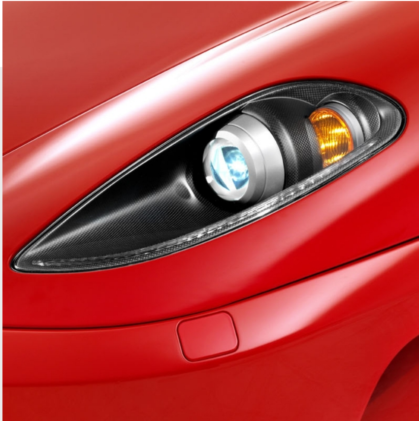
Carbon fibre headlamp tubs
