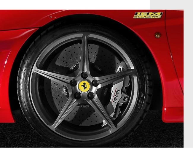
Using forged wheels reduces weight by 11 kg compared with standard wheels. A reduction in non-suspended mass guarantees a more direct feeling of contact with the vehicle, allowing customers with a more dynamic and demanding driving style to fully savour the sports spirit of their car.
