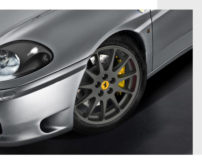
With a modern, sleek design, the multi-spoke wheel is offered in the original 18" wheel size for complete interchangeability with the original wheels and to avoid any possible problems regarding type approval. This solution also ensures that the vehicle configuration remains within the original design specifications for tyres, which is an indispensable prerequisite for safety and for the correct the ABS system to function correctly.
