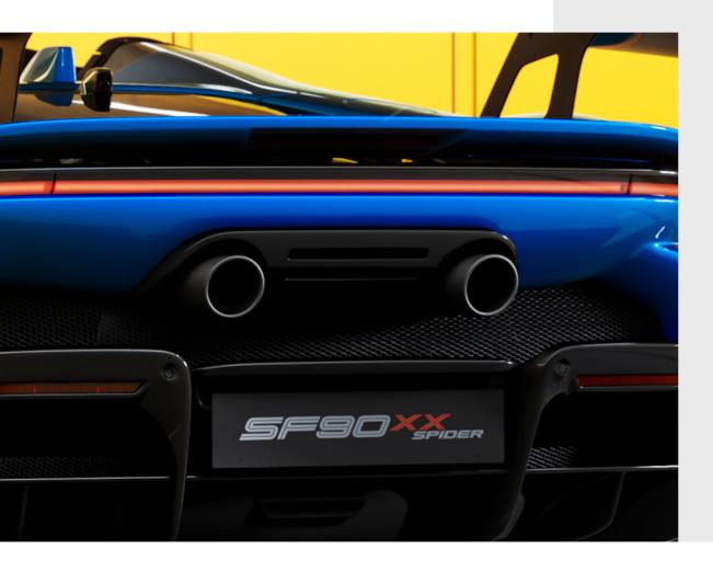
Designed on the same basis as the standard tailpipe tips, the titanium ones are 50% lighter and have a surface finish which helps them preserve the same appearance. Use of this technologically advanced material guarantees maximum resistance to external agents and is a perfect example of Ferrari's constant strive for product improvement.
