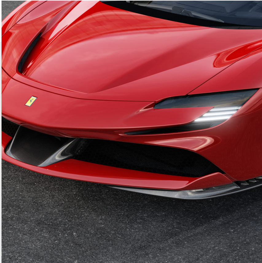
Carbon fiber front aerodynamic appendages
