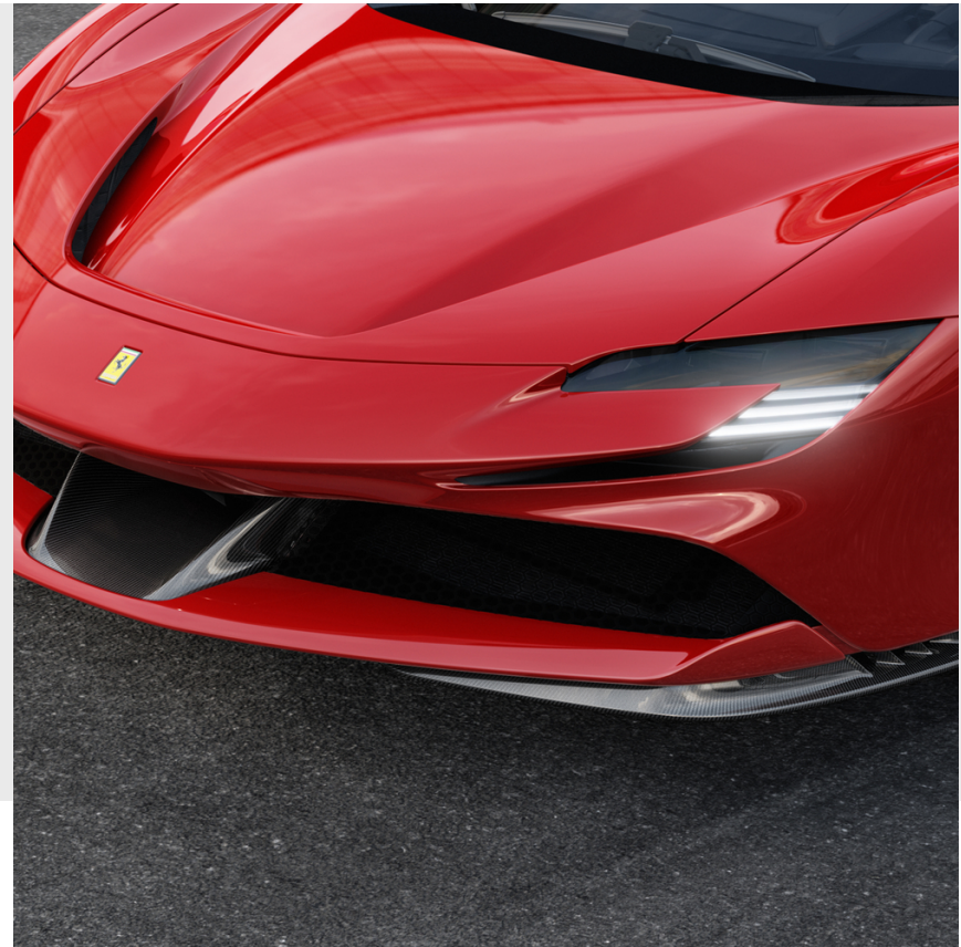
Carbon fiber front aerodynamic appendages
