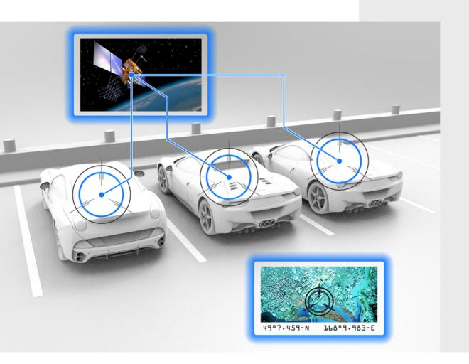
The Ferrari Genuine satellite alarm system is available in two versions, one with the ADR card and one without. The system with the ADR card recognizes the authorized driver by detecting the personal card (Automatic Driver Recognition), which is handed over to the customer when the anti-theft system is installed in the vehicle.
