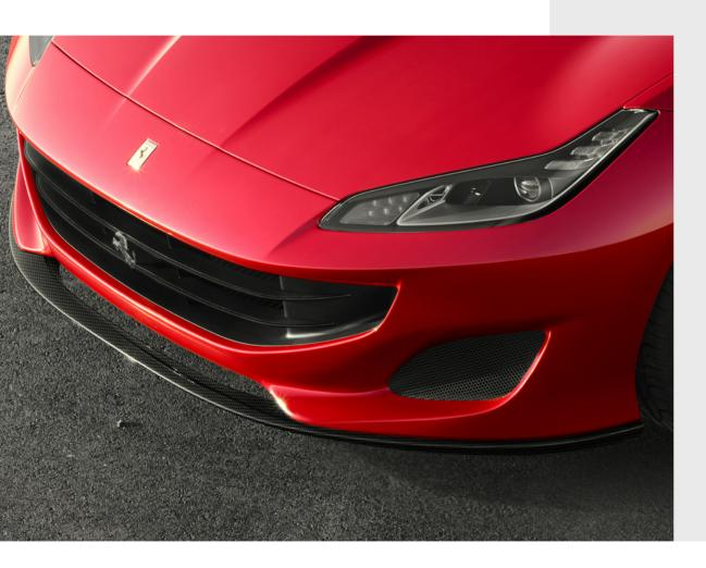
Developed with advanced fluid dynamics modeling technology and honed in the wind tunnel to optimize underbody aerodynamics, the carbon fiber front spoiler performs a crucial function for overall aerodynamic performance while offering the customer an opportunity to personalize the looks of their vehicle.
