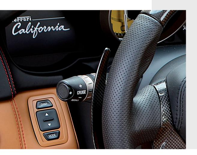
Cruise control is an electronic function that automatically maintains a constant speed when driving on long stretches of highway.
