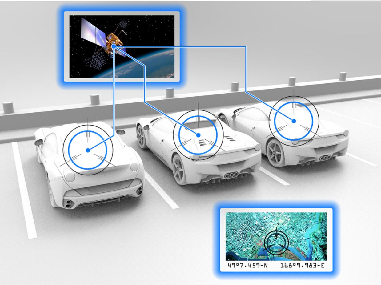
The Ferrari Genuine satellite alarm system is available in two versions, one with the ADR card and one without. The system with the ADR card recognizes the authorized driver by detecting the personal card (Automatic Driver Recognition), which is handed over to the customer when the anti-theft system is installed in the vehicle.
