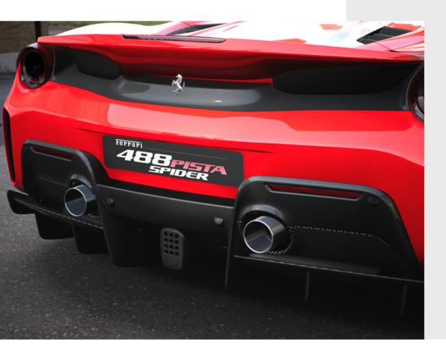
Designed to increase rear downforce and facilitate the evacuation of air from the underbody, the carbon fiber diffuser accentuates the style of the car while performing a precise aerodynamic function and contributing to reducing weight.
