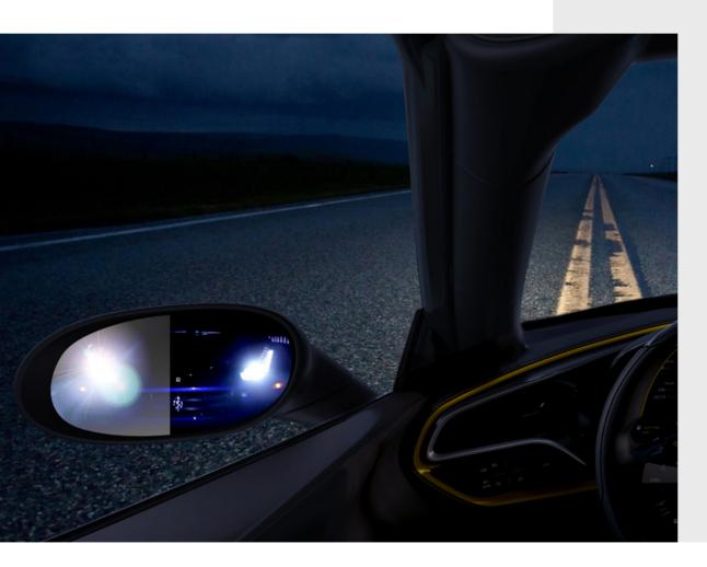
The electrochromic mirrors effectively reduce reflected glare for the driver. This mirror uses special electrochromic technology to darken quickly and automatically in response to the brightness of the light striking it.
