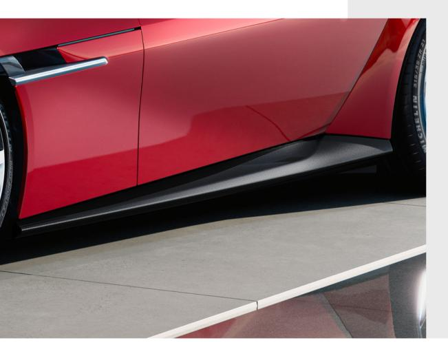
Ferrari Genuine gives customers the chance to replace the traditional under-door installed on the vehicle with an under-door kit in open weave carbon fiber.
