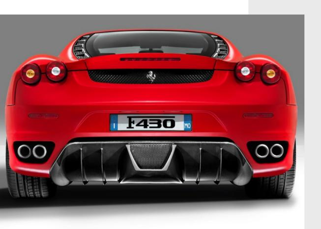
Designed to increase rear downforce and facilitate the evacuation of air from the underbody, the carbon fiber diffuser accentuates the style of the car while performing a precise aerodynamic function and contributing to reducing weight.
