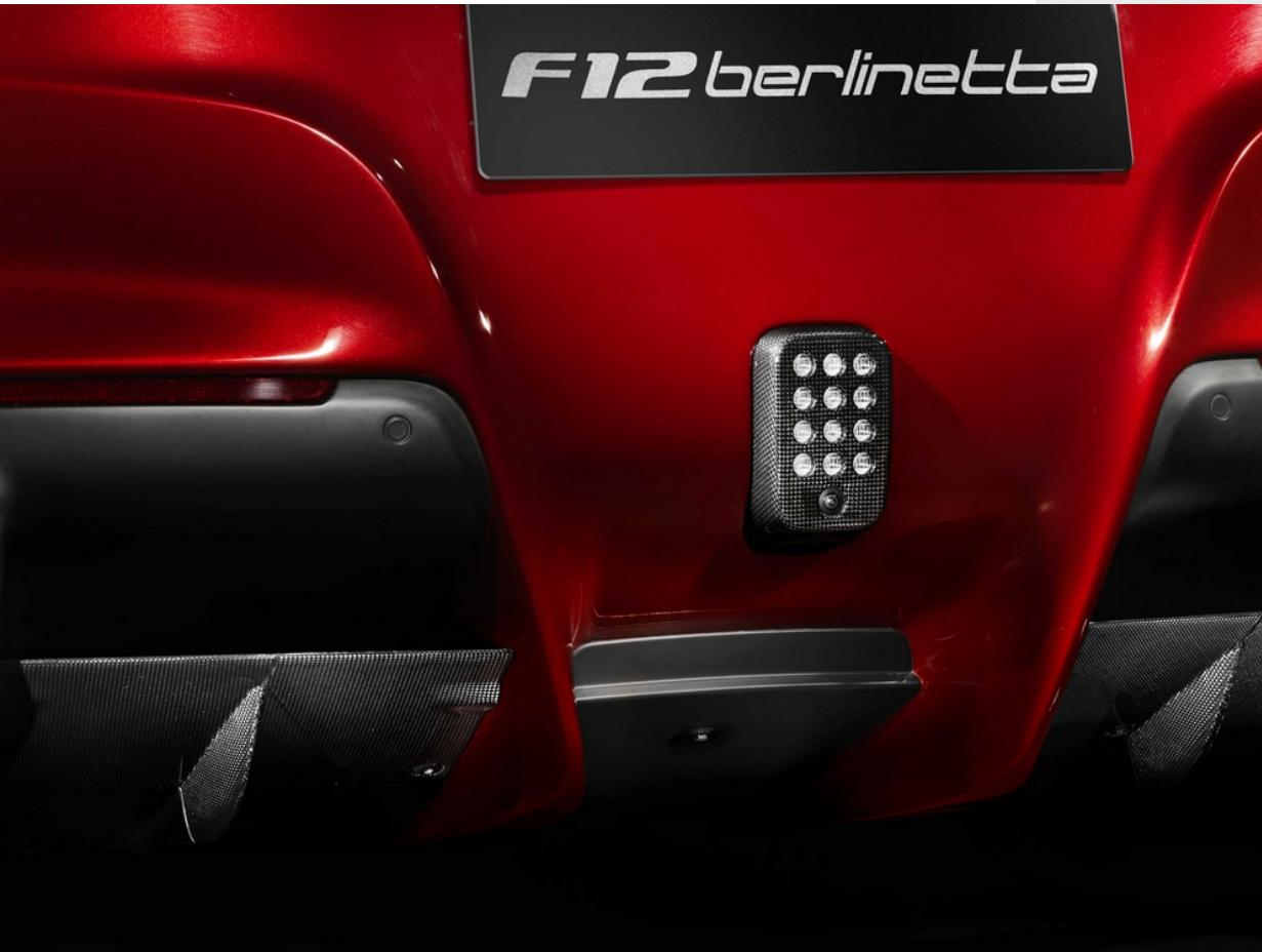
Designed to increase rear downforce and facilitate the evacuation of air from the underbody, the carbon fiber diffuser accentuates the style of the car while performing a precise aerodynamic function and contributing to reducing weight.
