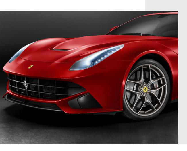
To guarantee a better driving experience as far as safety and performance are concerned, the Genuine accessories catalog offers customers the chance to install Advanced Frontlighting System (AFS) headlights which direct the beam according to the direction of the bend, optimizing the light intensity and improving visibility.
