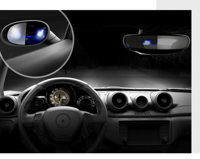
The electrochromic mirrors effectively reduce reflected glare for the driver. This mirror uses special electrochromic technology to darken quickly and automatically in response to the brightness of the light striking it.
