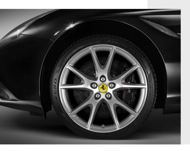
The 20" light alloy wheels enhance the vehicle's sporty character. The diameter enables tires with a smaller shoulder to be fitted which further enhance the vehicle's dynamic lines. The distinctive design, with five spokes split into twin branches, is a style feature that recalls GT championship wheels. The diamond finish gives the wheel a special sheen, shows off its shapes and forms, and gives the vehicle an extra touch of personality.
