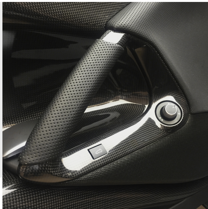
Internal door handles in carbon fiber, LH side
