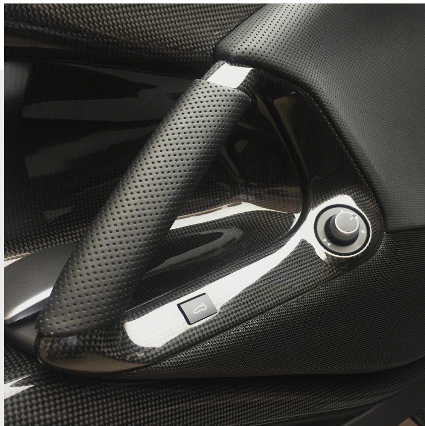
Internal door handles in carbon fiber, left with memory buttons
