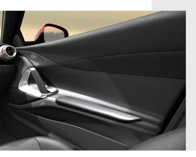
The carbon fiber door panels are an example of Ferrari excellence in the development of technological composite elements and help to enhance the sporty style of the passenger compartment.
