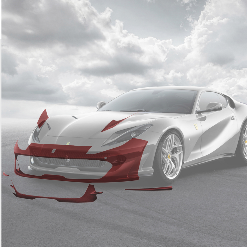
Anti-stone chipping protective film, front bumper
